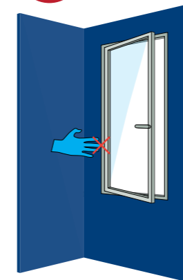
Risk of injury by getting stuck between window or door sash and frame.
