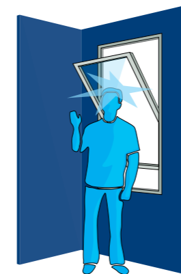
Risk of injury caused by sash impact.
