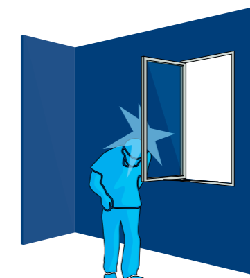
Risk of injury caused by sash impact when sashes are left open.
